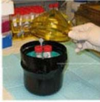
Always use sealed safety cups, safety buckets, or sealed rotors with O-ring as secondary containment.
